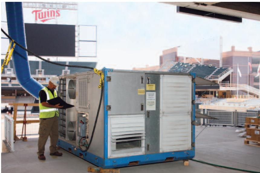
Temperature and relative humidity readings are collected by Polygon operations technician to determine performance of the HCU-6000.
